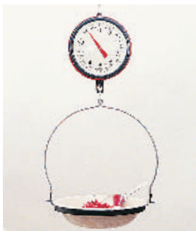
Figure 4 A spring scale is used to measure an object's weight.
